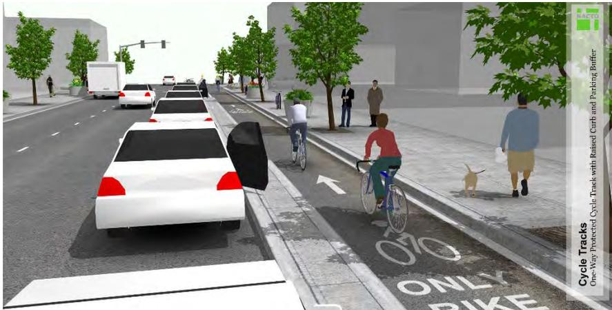
On-street bike lanes with a physical barrier separating the bike lane from motor vehicle traffic. The barrier can include flower planters, concrete curbs, plastic bollards, jersey barriers, and parked cars. Protected bike lanes can be either one-way or two-way.
