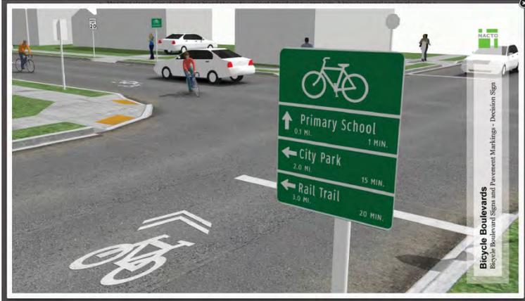
A bicycle wayfinding system consists of comprehensive signing and/or pavement markings to guide bicyclists to their destinations along preferred bicycle routes. Signs are typically placed at decision points along bicycle routes – typically at the intersection of two or more bikeways and at other key locations leading to and along bicycle routes.
