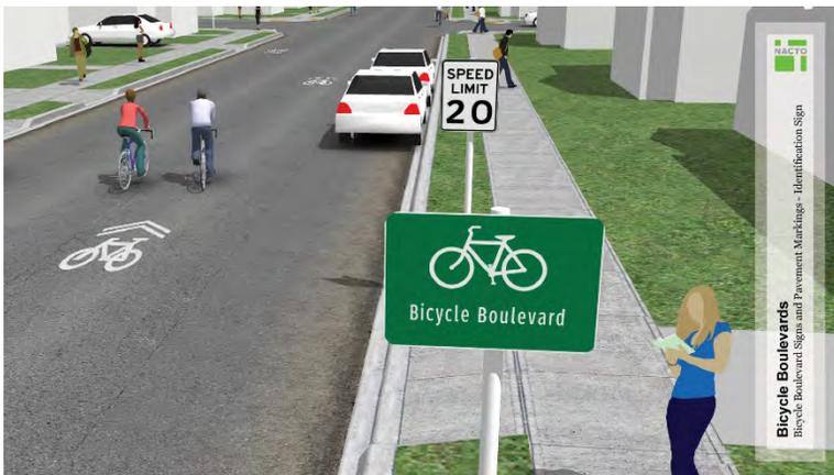
Bicycle boulevards are streets with low motorized traffic volumes and speeds, designated and designed to give bicycle travel priority. Bicycle Boulevards use signs, pavement markings, and speed and volume management measures to discourage through trips by motor vehicles and create safe, convenient bicycle crossings of busy arterial streets.
