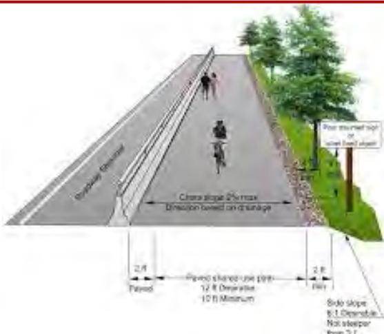
A multi-use pathway is physically separated from motor vehicle traffic, and can be either within the highway right-of-way or within an independent right-of-way. Multi-use pathways include bicycle paths, rail-trails or other facilities built for bicycle and pedestrian traffic. There should be a clearly defined origin and destination.
