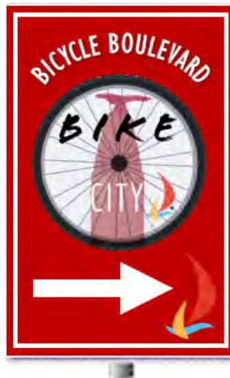
Indicates where a bikeway turns from one street onto another street. Can be used with pavement markings
