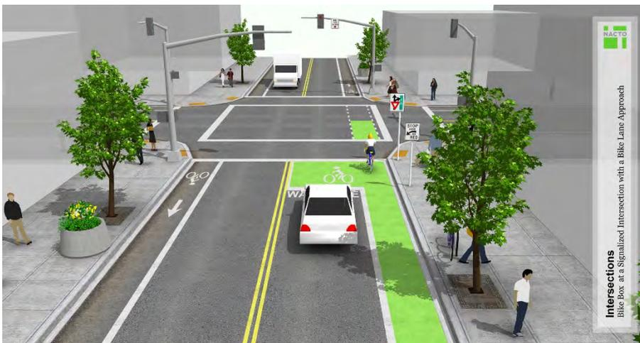
Green-painted rectangles (with a white outline) at intersections that provide a safe refuge for bicyclists to either cue ahead of cars or to make a two-stage turn. Bike boxes help increase safety for bicyclists by reducing right-hand hooks by cars and by helping bicyclists navigate tricky intersections, such as where there are streetcar tracks.
